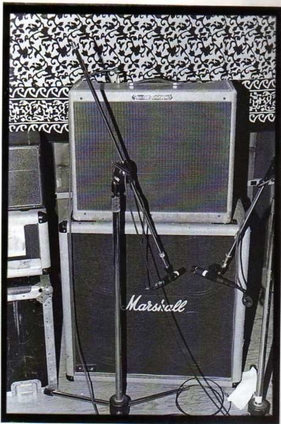
Robinson's Marshall Jubilee-series cab was close-miked using an AKG C-1000 and a Shure SM57 in an off-axis arrangement.
